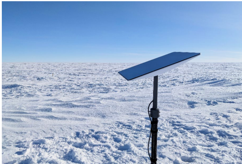
Figure 8: Starlink antenna in a short-term test at the SPRESSO site.
